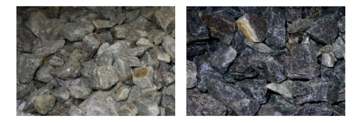
Sorting of -70 + 25 mm AHP. Lithium bearing pegmatite product (left) and amphibolite reject (right)
